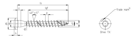
Power-Fast self-drilling screw - Wood connector screw with full thread
