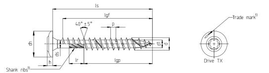
Power-Fast wood construction screw - Flange head with full- or partial thread
