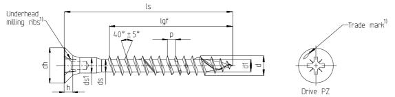
Power-Fast self-drilling screw - Countersunk headhole screw with full thread
