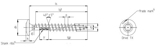
FCS wood construction screw - Flange head with partial thread
