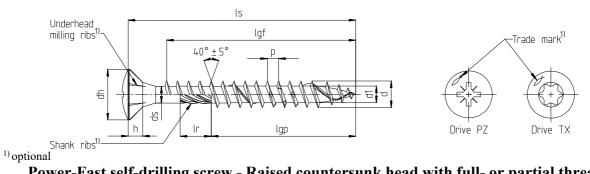
Power-Fast self-drilling screw - Raised countersunk head with full- or partial thread
