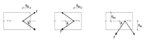
Definition of spacing, end and edge distances in the edge surface unless otherwise specified in the technical specification (ETA or hEN) for the cross laminated timber.
